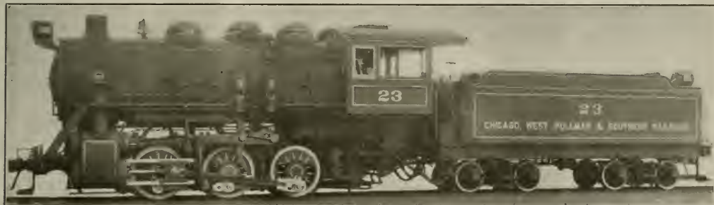
SIX-COUPLED SWITCHING LOCOMOTIVE FOR THE CHICAGO, WEST PULLMAN & SOUTHERN RAILROAD. BALDWIN LOCOMOTIVE WORKS, BUILDERS
